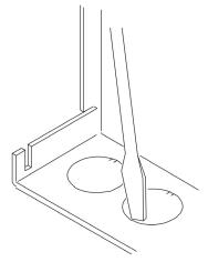
Remove the required knock-outs for cable entry.
